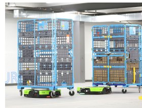
Fig. 1: Amazon’s Proteus robots [1] carry uniform loads and are example platforms that can be used for multi-robot ordered storage and retrieval in warehouses.
